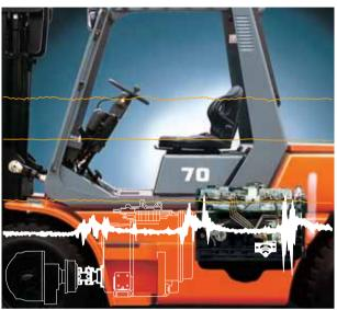
The 5-series uses a full-floating system that vastly reduces the amount of engine vibration transmitted to the frame, assuring a ride of unmatched comfort. This promises not only more comfort for the operator, but greater frame durability as well. At Toyota, advanced technology goes hand in hand with superior comfort. That is the concept of TECHNO-COMFORT the idea that the benefits of our ongoing technical development are ultimately for the operator.
